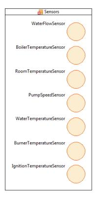
You are asked for names. Create a Channel for the WaterFlowSensor (F1), BoilerTemperatureSensor (T2), PumpSpeedSensor (S3), IgnitionTemperatureSensor (T4), BurnerTemperatureSensor (T5) WaterTemperatureSensor (T6) and there must be a RoomTemperatureSensor (T7).
