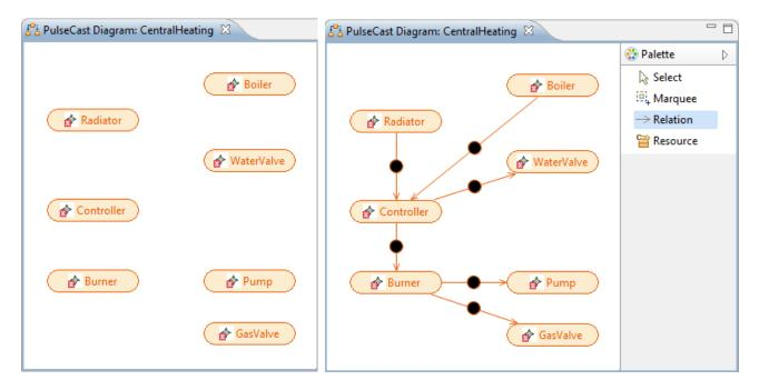
The connections are called Pulse Translations: A Pulse Translation connects an Outpulse of a Process to an Inpulse of another Process. You can open an Editor with a double-click on the bullet of a pulse cast.
