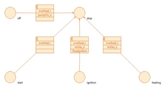
The overheat mode is controlled by the single state overheat in the Controller process. The mode changes the behavior of the process. But if there are actions to be done upon a mode switch, they must be modeled separately: Pulses sent in a transition, that causes a mode switch in the receiver process, is received already in the new mode.
